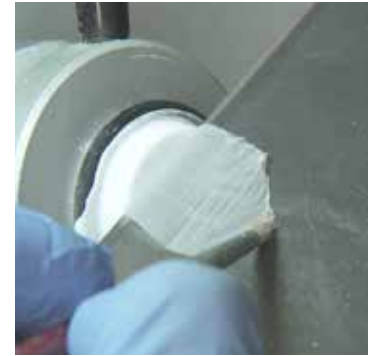
12. The slice is picked up by the slide and processed and stained with PRESTO.
