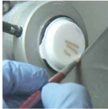
11. The specimens are now ready for cutting to obtain a perfect section, because of the planarity of the three specimens.
