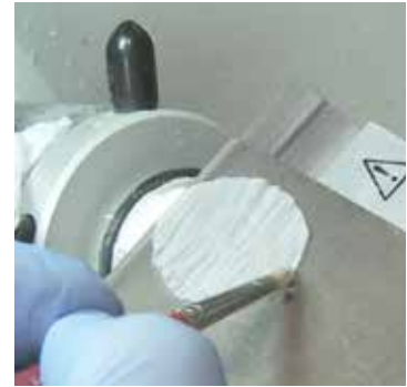
9. A section is prepared for picking up by slide.
