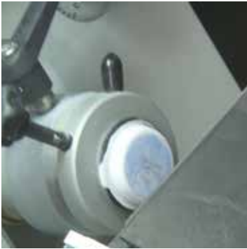
10. Place the chuck in the cryostat and trim the block until the paper is cut away.
