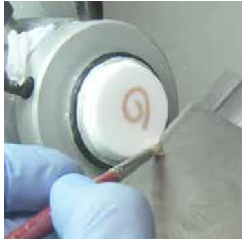
8. After trimming the paper away, the specimen is ready for cutting.
