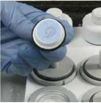
7. After 60 seconds the specimen chuck surface is ready and covered by the paper disk.
