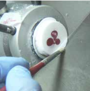
10. After trimming, the block is ready for sectioning.
